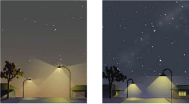
*The Master Plan recommends fixtures with a sharp cutoff to direct light downward to usable areas (right), as opposed to non cutoff light fixtures that create excess light pollution and waste energy by throwing light into the trees and sky (left)*
