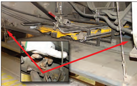
Figure 1-13 – Lower storage compartment latches and safety cables
