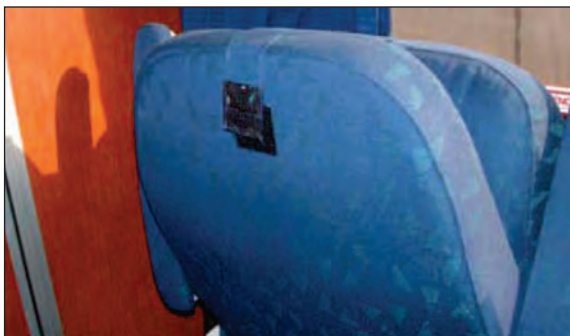
Figure 12-7 – Velcro Fabric Strap Securing Seat Cushion in Folded Position
