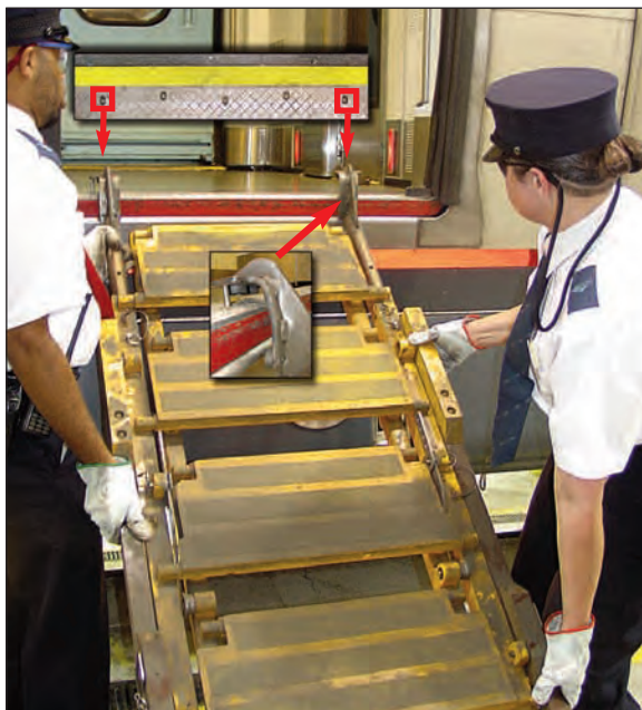
Figure 1-15 – Secure folding stairs to car body
