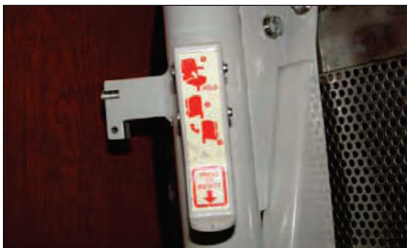
Figure 12-9 – Close-up View of the Foot Operated Latch Mechanism
