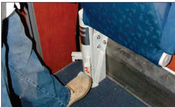
Figure 12-8 – Foot Operated Latch to Secure or Release the Bedroom Occasional Seat from Against the Wall
