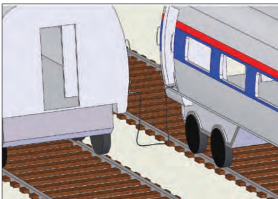
Figure 1-3 – Remove jumper cable from transfer bridge bag and connect to metal car body of both train cars involved in the transfer.
