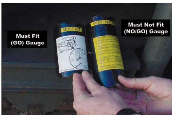
Figure 12-1 – Must Fit (GO) Gauge and Must Not Fit (No/Go) Gauge
