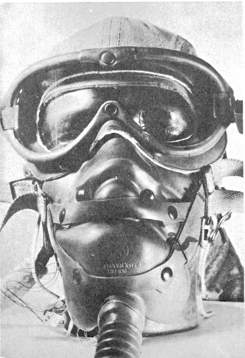
Figure 24 — Breathing Head . . . For Study of Freezing Conditions in Oxygen Mask
