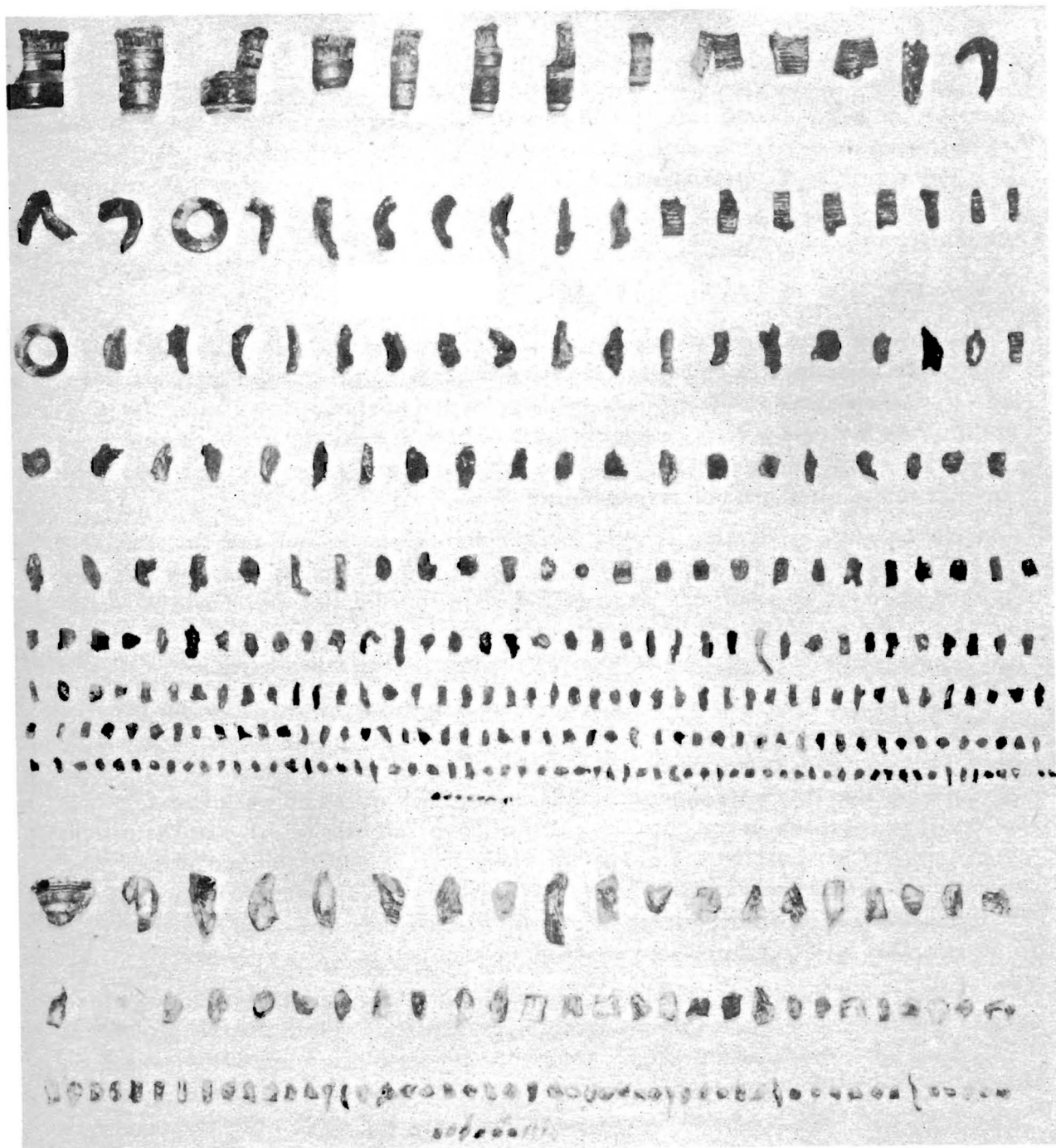
Figure 47 — Fragments of a Single German 20 mm HE Explosive (60% Actual Size)
