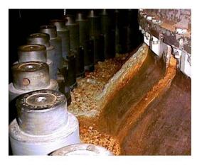
Pictures taken in 12RFO of the reactor vessel head flange showing boric acid with rust diffusion out of the ween holes.
