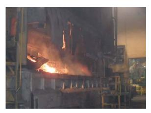
Furnace used for melting aluminum
