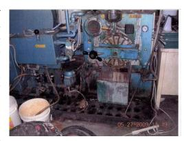
Equipment with hose draining PERC into bucket
