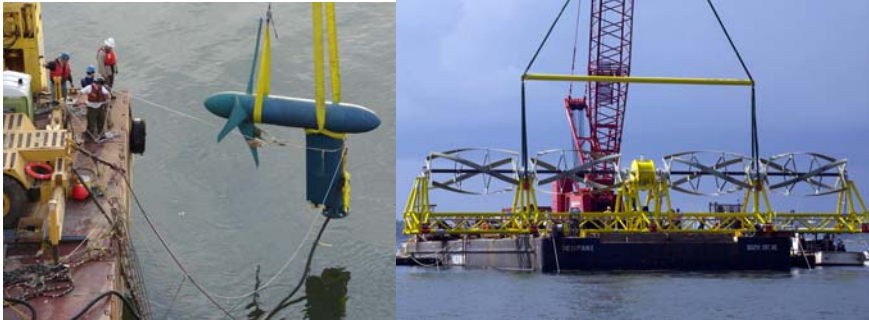
Figure III-6. (Left) Verdant Power's axial-flow turbine CEC, similar in design to today's commercial-scale wind turbines, being deployed in the East River near New York City [21]. (Right) A cross-flow turbine developed by Ocean Renewable Power Company being prepared for an open water test [22].
