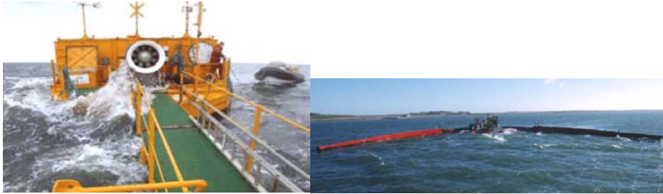
Figure III-5. (Left) Ocean Energy Limited's AWS oscillating water column device showing the air turbine that is used to generate energy. (Right) The Wave Dragon overtopping device undergoing open-ocean testing.
