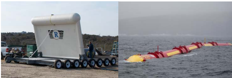
Figure III-4. (Left) Resolute Marine's terminator prototype being prepared for a test deployment, courtesy of Resolute Marine Energy. (Right) Aquamarine's Pelamis attenuator device in open-ocean testing, courtesy of Pelamis Wave Power.
