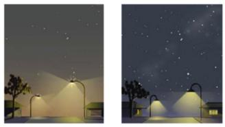
The Master Plan recommends fixtures with a sharp cutoff to direct light downward to usable areas (right), as opposed to non cutoff light fixtures that create excess light pollution and waste energy by throwing light into the trees and sky (left)
