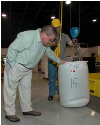
PHMSA Packaging Program Manager Anthony Lima (lt) and LOGSA Engineer Ben Moore (rt) examine a UN standard plastic drum after a successful five-foot drop test.
