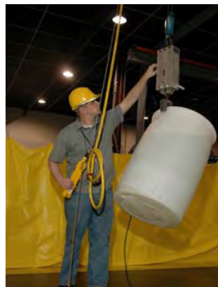
LOGSA Engineer Ben Moore prepares to conduct a drop test on a UN standard plastic drum.
