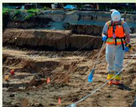
Figure 2 - DNMS inspector Daniel Strohmeyer conducts radiation surveys at Hematite facility using Ludlum 44-10 NaI 2x2 gamma detector coupled with Trimble GPS instrument.
