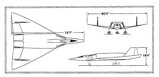
important design features that contributed to a small radar return were fiberglass engine inlets and wings whose leading edges were made of Pyroceram.<sup>14</sup>
