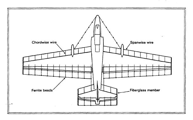
absorption devices for the U-2. Once these devices were installed on the operational U-2s, he explained, the "majority of incidents would be undetected." <sup>73</sup>
