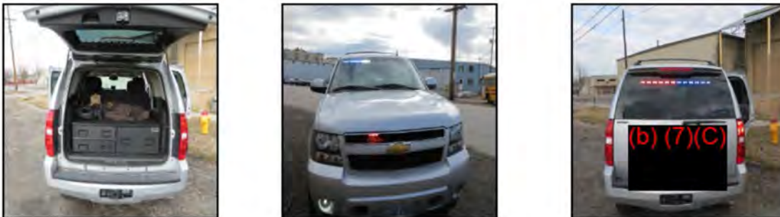
Figure 2. Interior space of the vehicle and rear wig-wag and emergency flashing lights added to (b) (7)(C) Tahoe.
