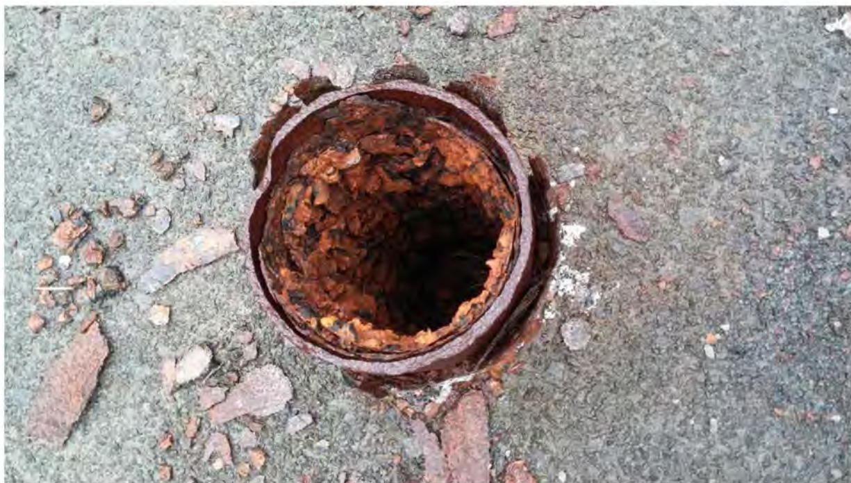
Figure 2. An example of a tuberculated pipe at the park, although this particular pipe was not in use. Source: OIG.
