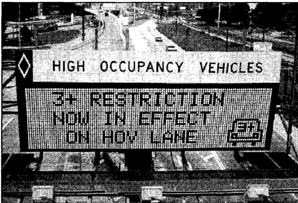
Figure 6-30. Example of Dynamic Message Sign Showing New Occupancy Requirement.<sup>(9)</sup>
