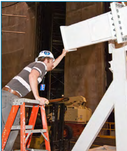
Lead engineer Steve Sinclair inspects the massive lifting fixture before moving a shroud panel. The structure is comprised of panels and support beams.
