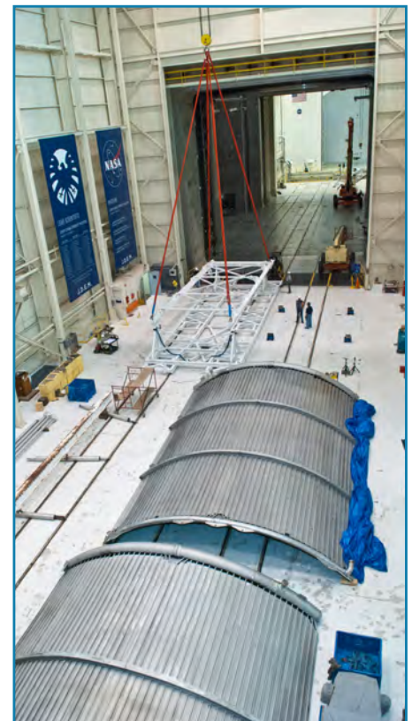
The facility team prepares for lifting a 40-foot-long shroud panel. The team's ingenuity allowed them to modify existing hardware instead of starting from scratch.
