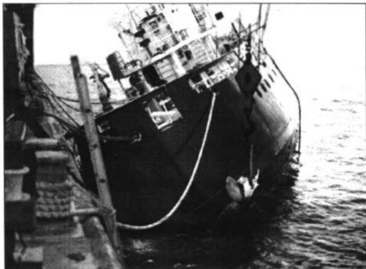
Figure 3-13. Propeller Being removed from the Wreck.
