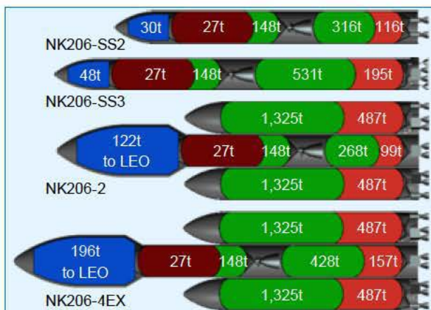
Figure 4-2 NK206 Family Tank Layout
