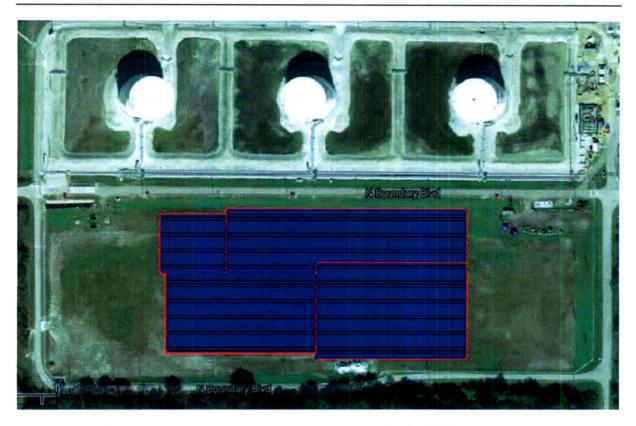
The total power production if all the phases are installed is 1,712,440 watts DC for power production of 2,461,352 kWh AC. The annual power production for all three phases was calculated using NREL's PV Watts modeling software using a derate factor of 0.81. Power production outputs for each phase are included in **Appendix D**.
