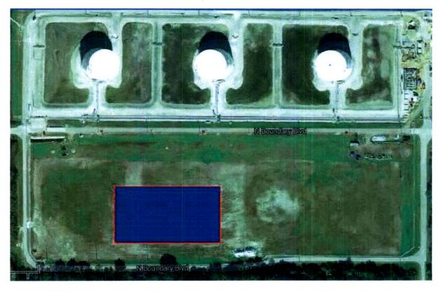
The second phase can be expanded an additional1,247,440 W DC producing 1,792,991 kWh AC. The following figure shows the proposed layout of the solar system for the second phase.
