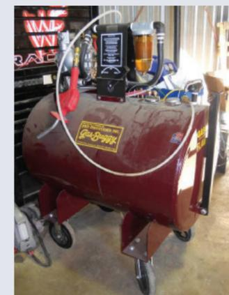
Waste fuel removal pump and containment tank.
