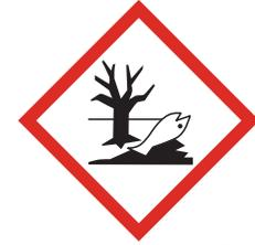
**Environmental Hazard:** Refrigerants may contain ozone-depleting substances and should not be vented into the air.
