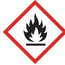
**Worker Hazard:** Refrigerants are gases under pressure and may be flammable.
