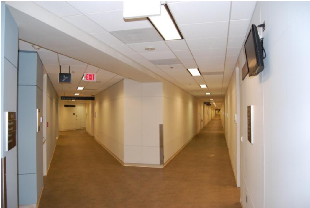
Figure 78 - Typical corridors (Source: QEA, 2013). Floor, wall, and ceiling finishes are not original.
