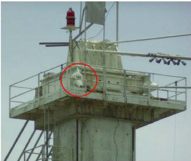
Figure 5. Failed clevis (circled). Photo from AO.
