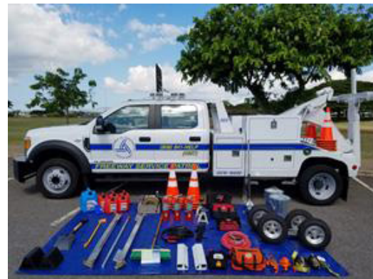
Figure 7. Photo. Safety service patrol vehicle and the equipment it carries.
