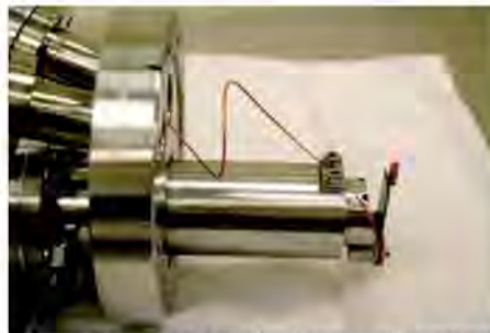
FIGURE 1. X-ray beam shutter. Shown are the piezo bender, copper shim and stainless steel stanchion.
