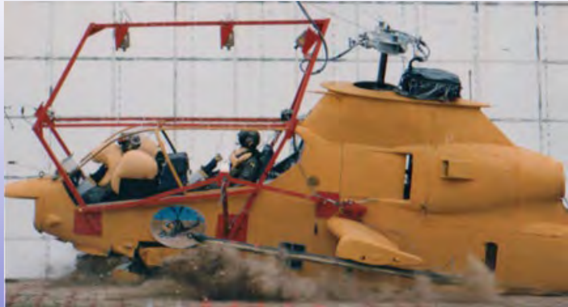
Crew Airbag System (CABS) and Inflatable Body and Head Restraint System (IBAHR)
