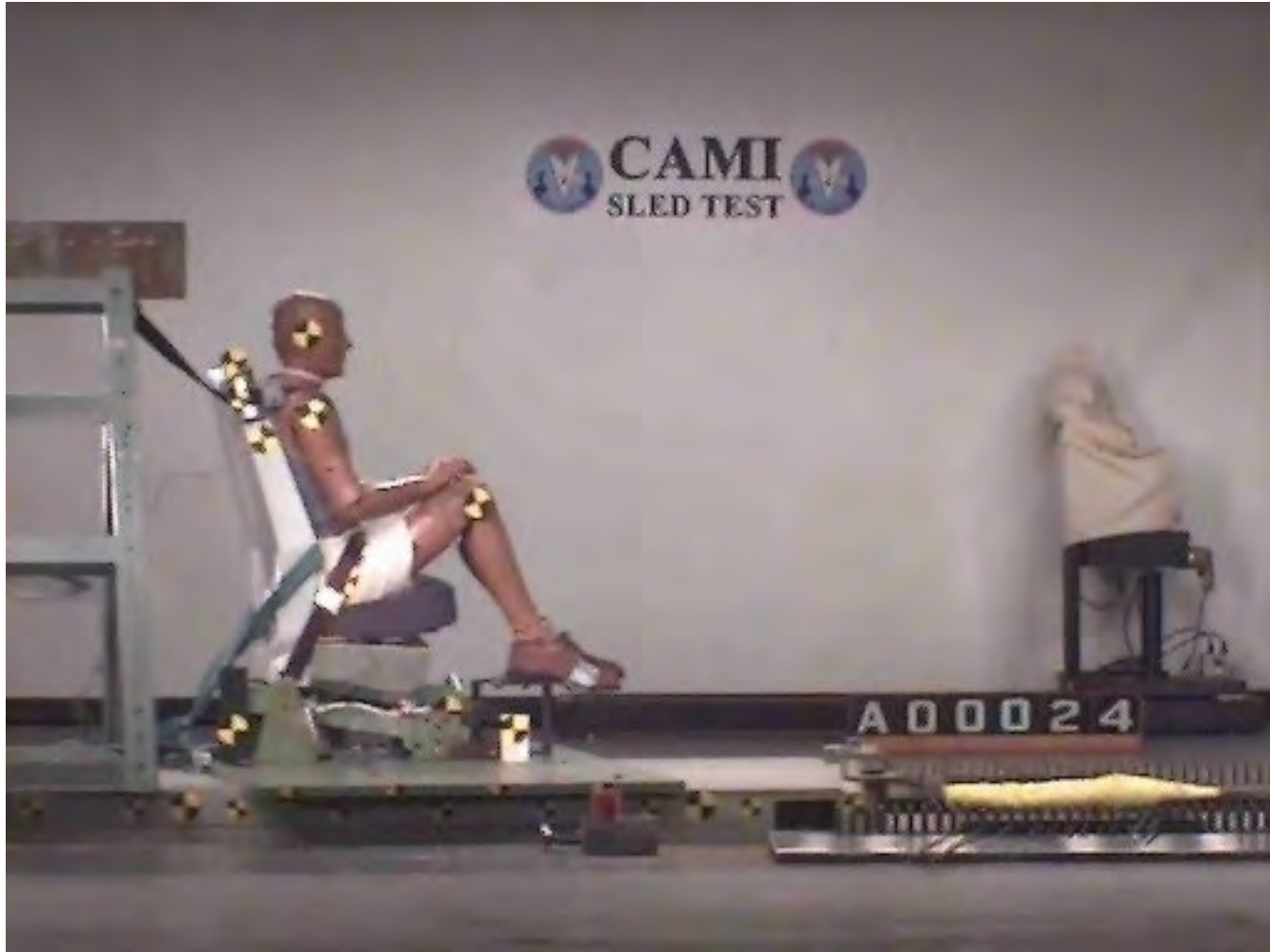
Part 23 Horizontal 21 G Passenger Seat
