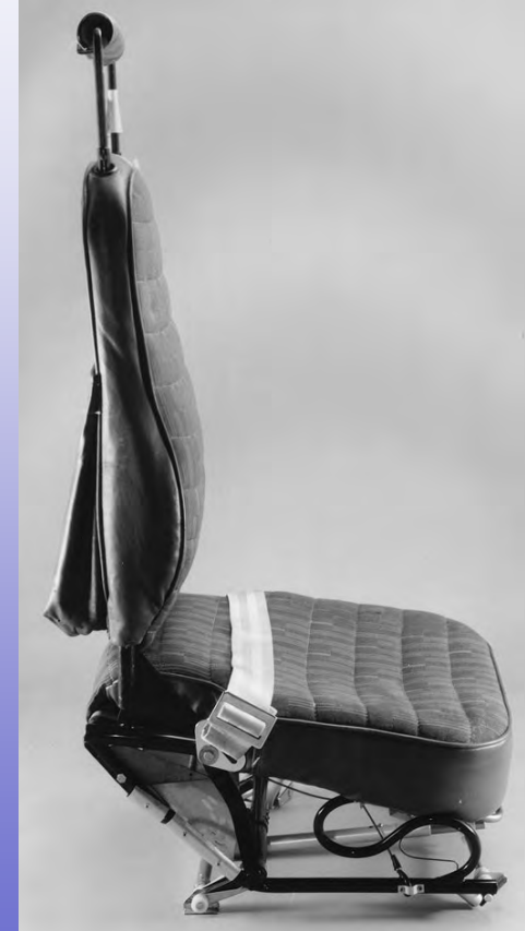
JAARS Energy Absorbing Seat Post-Test
