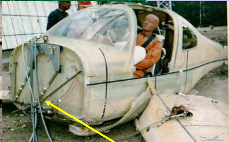
Failed Engine Mount
