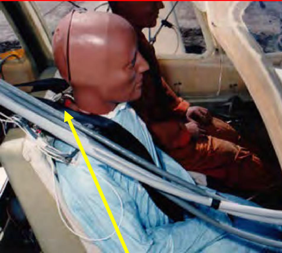
Shoulder harness restraint attached to aircraft structure
