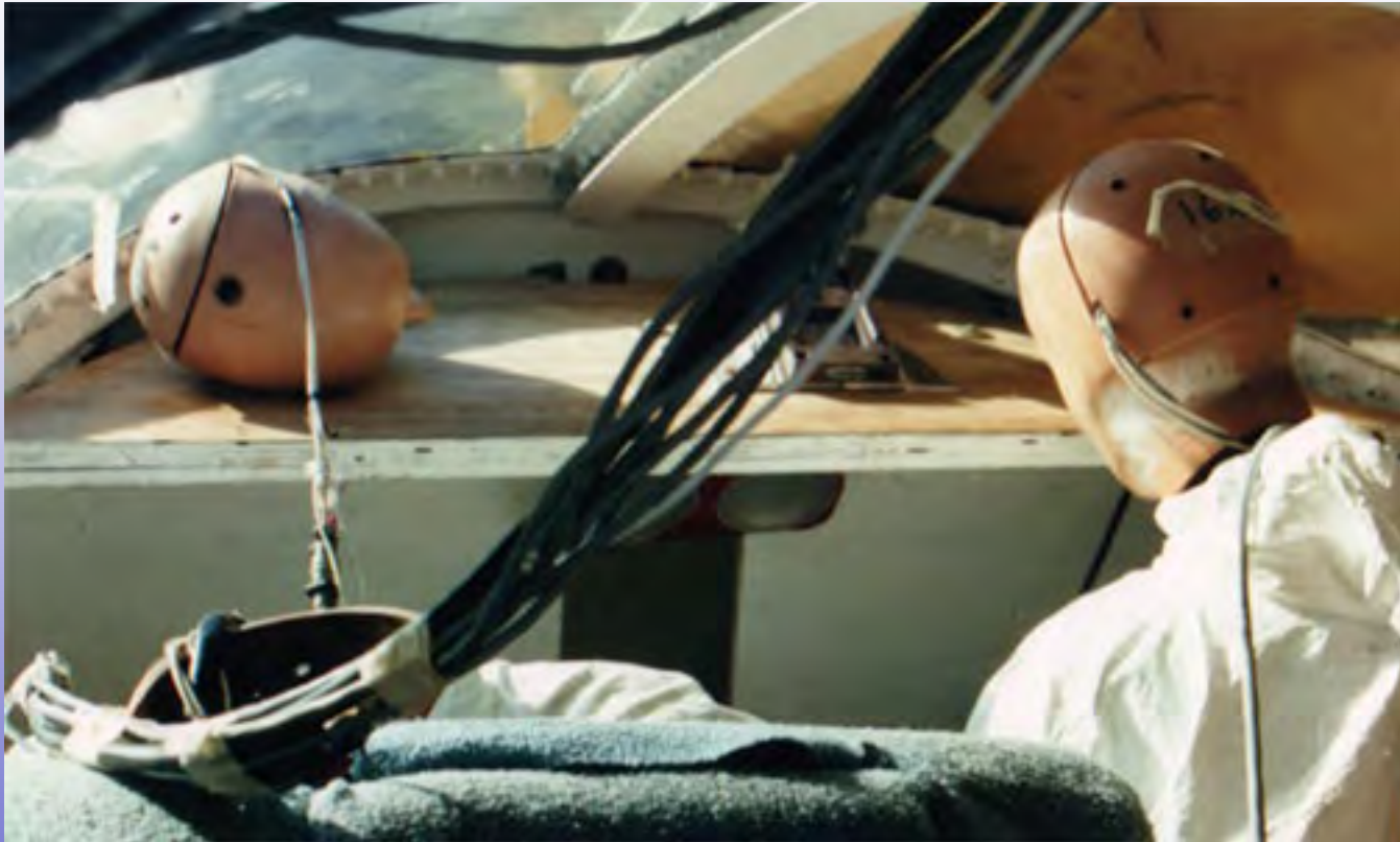
Pilot with lapbelt only allowed head strike
