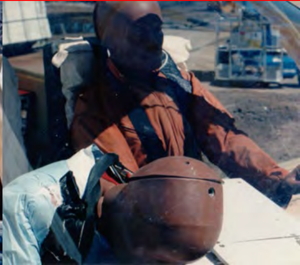
Attachment to aircraft structure fails allowing head strike
