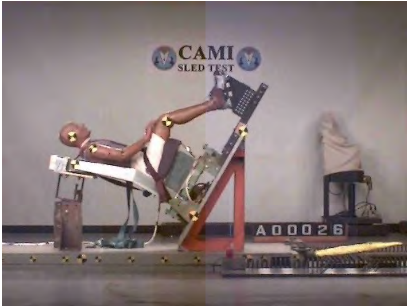
Part 23 Vertical 19 G Passenger Seat
