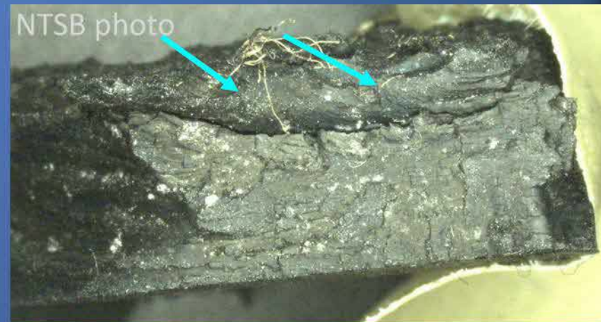
Tread Rubber Reversion An oval-shaped area in the tread similar to a skid, but where rubber shows burning due to hydroplaning during landing usually caused by wet or ice-covered runways. Remove if balance is affected.
