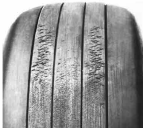
Chevron Cutting Tread damage caused by running and/or braking on cross-grooved runways. Remove if chunking to fabric occurs or tread cut removal criteria are exceeded.
