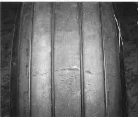
Open Tread Splice A crack in the tread rubber where the joint (splice) separates in a radial (sideways) direction. Tires with this defect should be removed from service.
