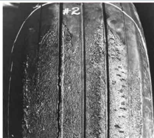
Tread Rubber Reversion An oval-shaped area in the tread similar to a skid, but where rubber shows burning due to hydroplaning during landing usually caused by wet or ice-covered runways. Remove if balance is affected.
