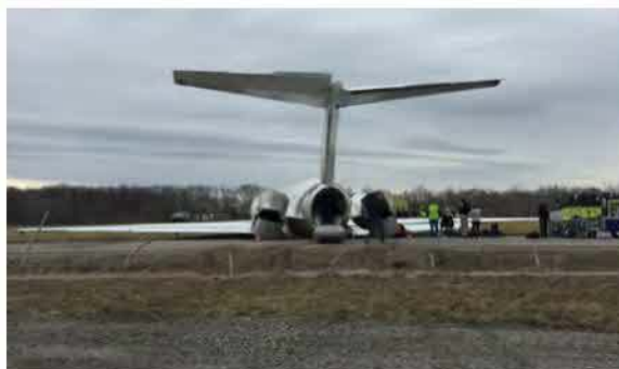
Figure 17. The probable cause of the runway overrun of this Boeing MD-83 airplane was a jammed right elevator resulting from strong, turbulent wind gusts.
