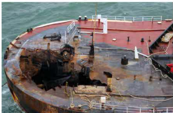
Figure 32. The B. No. 255 sustained significant bow damage from the explosion.
