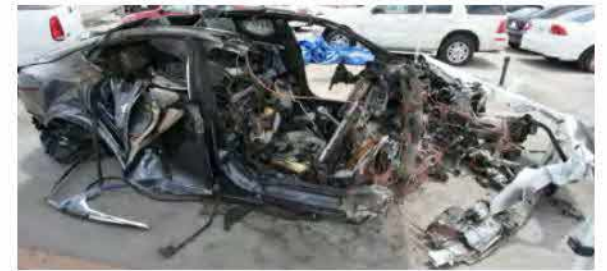
Figure 28. The right side of the car involved in the Fort Lauderdale, Florida, accident, shows the severe crash and fire damage.
