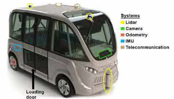
Figure 27. The external sensors and communication devices that guided the autonomous shuttle in the Las Vegas accident were located on the vehicle as shown below.
