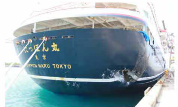
Figure 38. This close-up of the starboard side of the stern of the MV Nippon Maru shows the damage to the ship.
