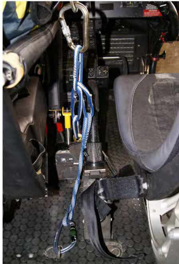
Figure 20. This photo shows the front passenger's tether with top locking carabiner inserted through the third webbing loop (from floor) with three excess loops hanging as a tail. Note: The tether tail's terminating loop (yellow) is partially obscured.
