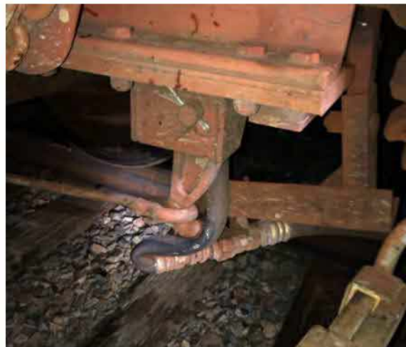
Figure 54. The November 2018 train collision in Granite Canyon, Wyoming, killed 2 crewmembers and derailed 3 locomotives and 66 railcars. This picture shows damage to the brake rigging of one of the railcars.
