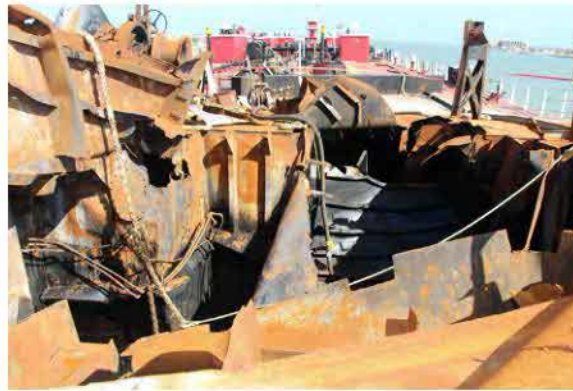
Figure 33. Looking aft from barge B. No. 255 , the damage to the chain locker, center forepeak and port forepeak ballast tanks is visible.
