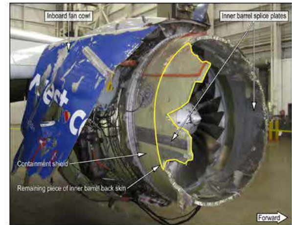
Figure 21. The engine inlet of the Boeing 737-700 was substantially damaged when the inner barrel forward of the containment shield separated circumferentially from the rest of the inlet. Only a portion of the inner barrel back skin remained.
