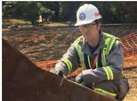
Figure 56. Frank Zakar of the Materials Laboratory Division examines the pipeline fracture in Danville, Kentucky.
