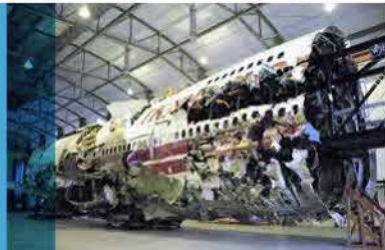
Figure 61. Weighing about 60,000 pounds and consisting of almost 1,600 pieces, the 93-foot section of the center fuselage of TWA flight 800 was transported to and reassembled at the NTSB Training Center in 2003. Since then, it has been used to train thousands of investigators from around the world.
