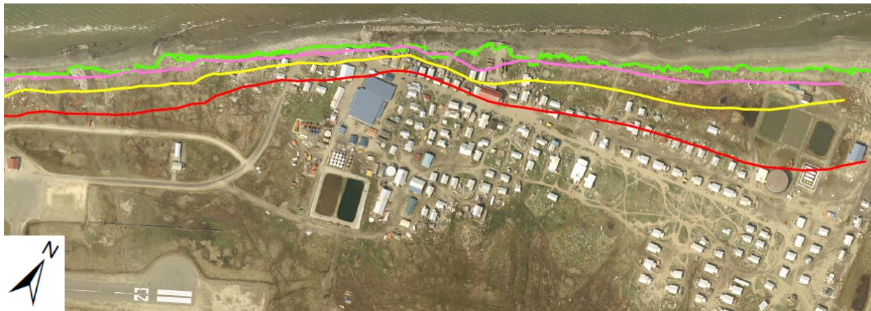
Figure 3-1. Shishmaref, Alaska, erosion prediction assuming no coastal protection.
