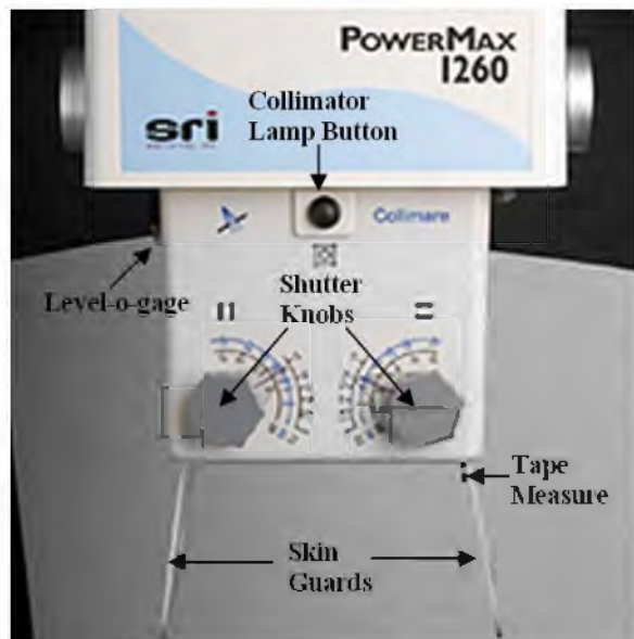
Figure 7. X-ray Generator Description.
