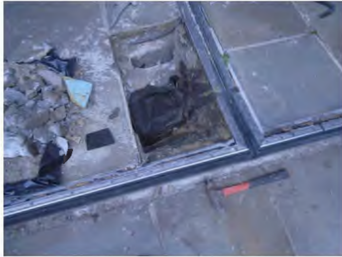
Photo Seal-2: Test Cut (TC2) at displaced expansion joint in Loading Dock area. Exposed curb was sounded with a hammer and found “unsound.”
