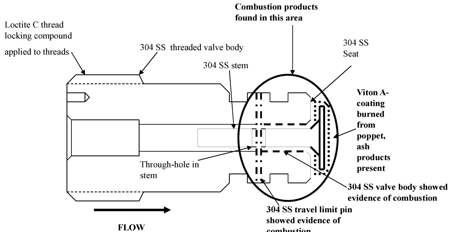
NOTE: During filling, stem moves back and forth due to pulsing action of pump. Captured pin in larger through-hole in stem limits travel.
