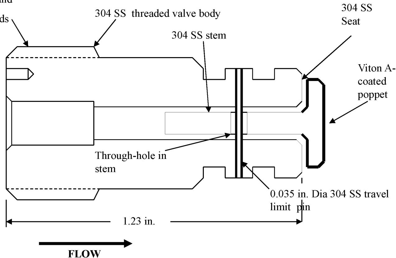
NOTE: During filling, stem moves back and forth due to pulsing action of pump. Captured pin in larger through-hole in stem limits travel.
