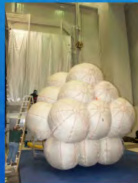
Mars Exploration Rover airbags: vectran bags strapped together
