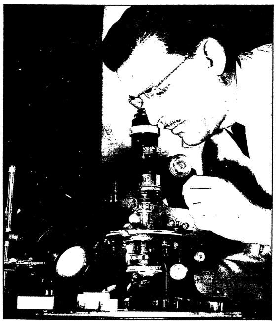
A LABORATORY TECHNICIAN USING THE PETROGRAPHIC MICROSCOPE FOR SOIL AND DIRT EXAMINATION, TECHNICAL LABORATORY, FEDERAL BUREAU OF INVESTIGATION, UNITED STATES DEPARTMENT OF JUSTICE.
