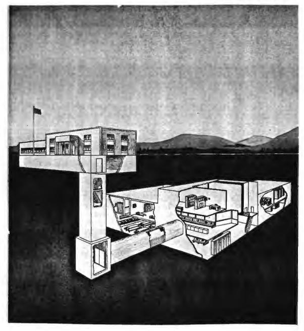
THIS IS AN ARTIST'S CONCEPTION OF THE UNDERGROUND COC AS PROPOSED BY CONAD/ADC IN 1956. BASED ON THE DESIGN FOR SAC, PROPOSED FACILITIES INCLUDED AN ABOVE-GROUND HEADQUARTERS, A BASEMENT, AND A THREE-STORY UNDERGROUND COC
