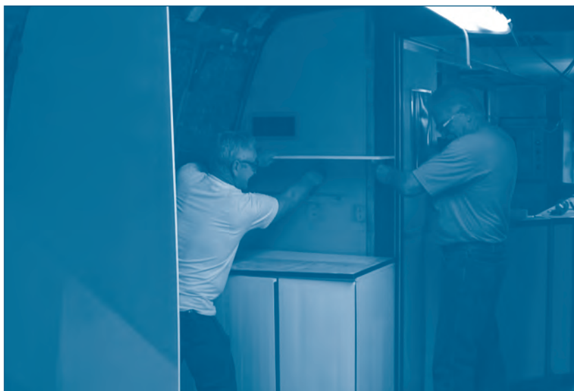
Working in the food preparation area, Car Repairman Cliff Bailey (left) and Sheet Metal Worker Jim Campbell determine the size and location for a mock-up shelf.
