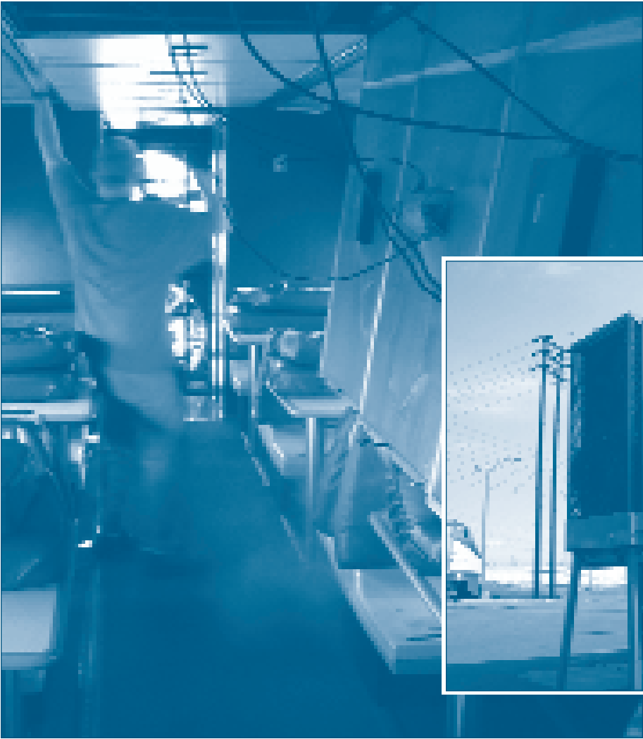
Carman Lance Johnson removes the ceiling panels in the Superliner Dining car while readying the car for preventive maintenance at Los Angeles 8th Street Yard. The wind machine (right photo) attached to the rear opening of the car, is then used to blow all dirt and debris out of the car using compressed air.
