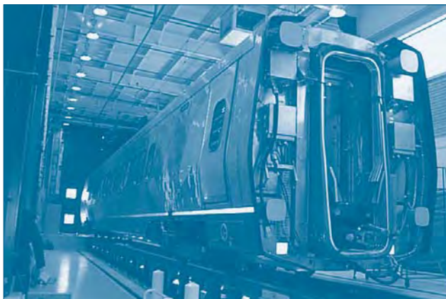
The AMTK10003 car is part of an Acela Express train consist, dedicated solely to track testing. Technicians use the instrument and testing area to edit and publish information as it comes off the car's systems, and railroad supervisors learn the condition of their railroad and review data that show areas that need repair.
