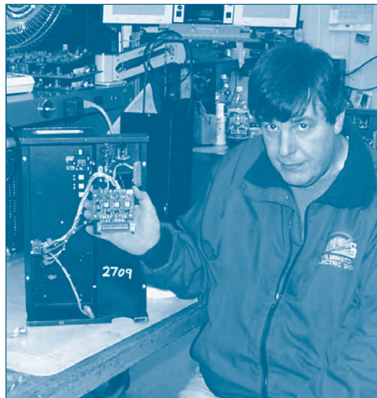
Bill Judefind, an electronic technician at the Wilmington Maintenance Facility, is shown with his newly-developed protection module boards that prevent the Public Address units from burning out.
