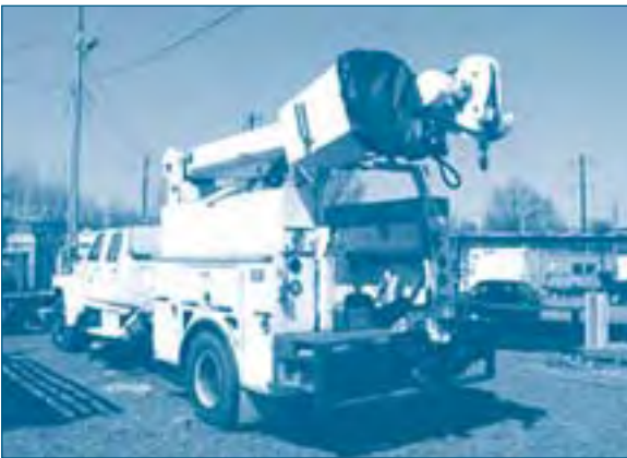
This three-man line truck features a 42-foot boom, an auger for digging poles, and a pole claw for loading poles. The five-year procurement vehicle replacement plan includes the purchase of eight boom trucks.
