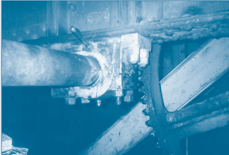
This deteriorated bearing and shaft, a component of the machinery that drives the Niantic River Bridge up and down, contributed to the inoperability of the bridge.
