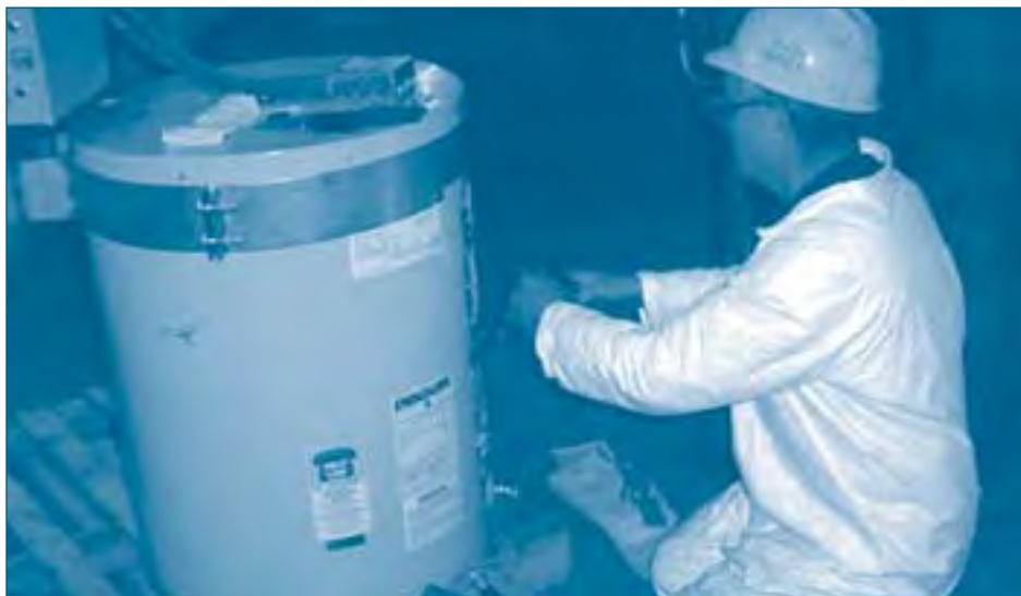
Jack Fund , electrician at Beech Grove, works on the heating elements of an A. O. Smith style water heater that will be installed into one of the wrecked Superliner cars.
