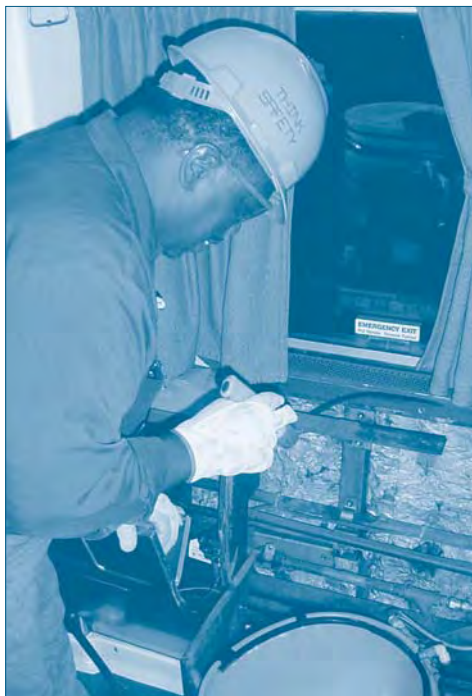
Mechanic Leroy Moore repairs the commode in Superliner Sleeping car 32002 as part of the car's 92-day inspection.
