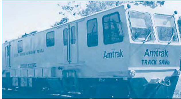
Amtrak's Track Structure Assessment Vehicle (TSAVe) is a self-propelled track geometry survey vehicle with GRMS (Gauge Restraint Measuring System) capabilities as its primary mission.
