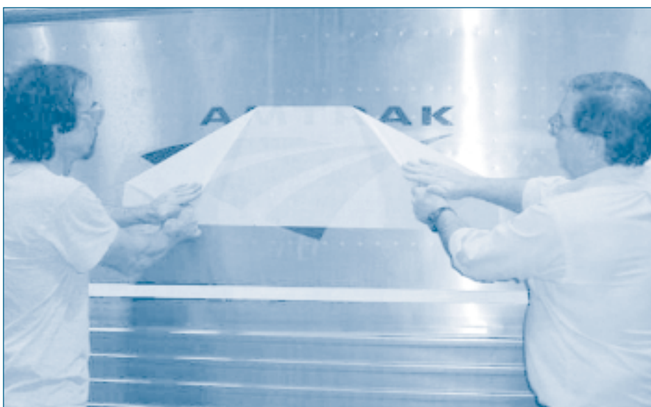
After applying the logo to Superliner II Sleeping car 32090, Carman Steve Anderson and Lead Carman David Riordan remove the application tape from the decal.
