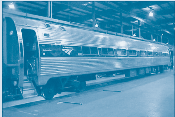
Metroliner Coach 21908 is the first wreck-repaired car that Bear Car Shop mechanics returned to revenue service this fiscal year. As a result of an October collision at Sunnyside Yards, the car sustained damage to the corner post, step, and door frame. The car was returned to service Nov. 19.
