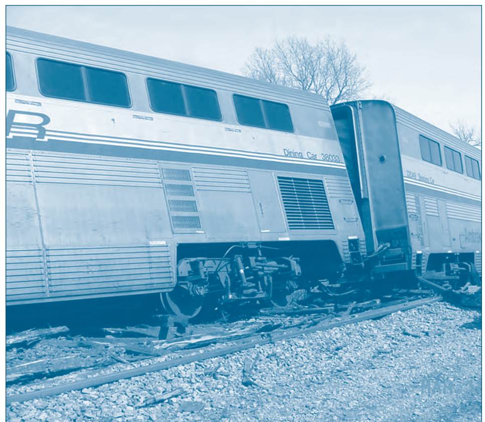
Superliner Diner car #38033, sits on the tracks tilted at a 15-degree angle as a result of the March 18, 2001, derailment of the California Zephyr in Nodaway, IA.
