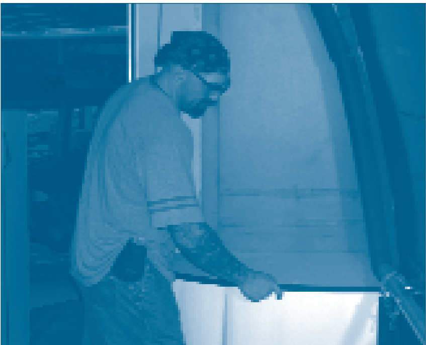
Car Repairman Chuck Ballard positions the foam board mock-up condiment station against the wall of the diner/lounge car. Mock-up components are used to develop engineering drawings so that the actual components can be built and installed.
